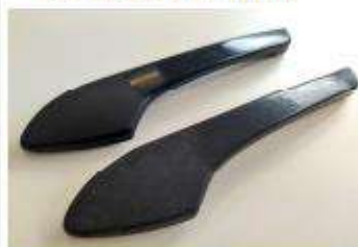
Door handle: recycled compound of 50% r-ABS and 50% composite CF of GF/Elium®
