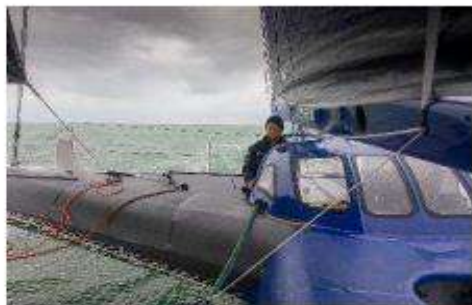
CFRTP: Aerodynamics fairing & roof with recycled Elium
