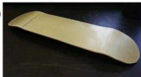
Fig. 10. A prototypical skateboard fabricated in part by thermoforming an Elium glass fiber and panel as reinforcement.
